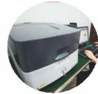
Energy dispersive X-ray fluorescence spectrometer To detect the harmful materials, according to the demand of EU standard
