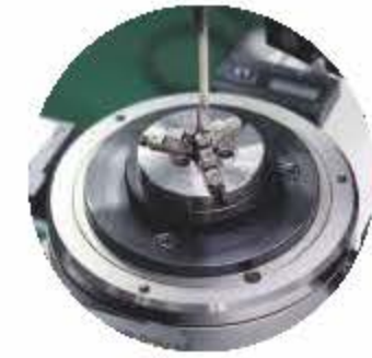
Roundness measuring instrument Imported from Japan, high degree of accuracy(0.01 um)
