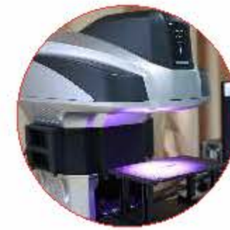
Profile gauge Imported from Japan For 3D measurement of precision parts
