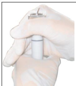
Picture 2: Fasten the scaling tip by wrench with the hand between thumb and index finger.
